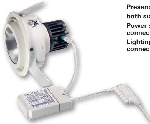
Downlight Primary side mains voltage, secondary side low voltage (SELV) Power supply system with gesis® MICRO code 1, white, for 230 V Lighting side with gesis® MICRO code 2, light blue, up to 50 V
