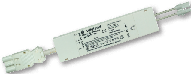
Electronic transformer Primary side mains voltage, secondary side low voltage (SELV) Power supply system with GST18i3 Lighting side with ST16 2-pole low voltage
