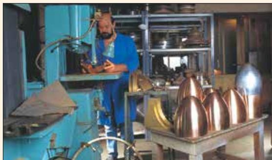
1 - After having diamond-cut the optical glass, the glassmaker adjusts each element in the bronze structure to perfection.
